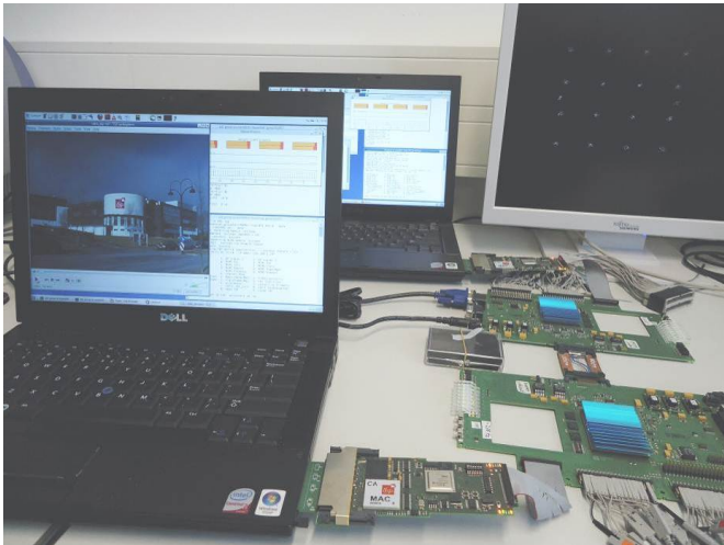
Figure 9. Photo of a system assembling the MAC and baseband boards
