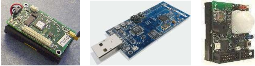
Figure 2. Current sensor node hardware: Mica 2 by Crossbow, Berkeley [26]; Tmote sky by moteiv, Berkeley [31]; and Embedded Sensor Board by ScatterWeb, Berlin [10]
