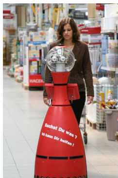
Fig. 1. Interactive mobile shopping assistant based on a SCITOS A5 platform developed by MetraLabs GmbH Ilmenau, Germany, during a guided tour to a goods location in our test site, an ordinary home improvement store in Erfurt (Germany).
