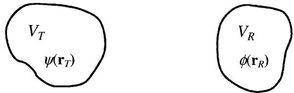
Fig. 2. Schematic diagram of the transmitting volume V_T , which contains sources \Psi(\mathbf{r}_T) of waves, and the receiving volume V_R , which contains a wave field \phi(\mathbf{r}_R) that arises from the sources in the transmitting volume.
