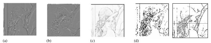
Figure 6: Horizontal(a) and vertical (b)Wavelet Transform, Wavelet Transform Modulus (c), Wavelet Transform Modulus Maxima above a given Threshold (d) and first center of gravity of lena.jpg (e)
