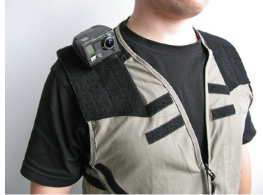
FIGURE 1: Wearable camera recording prototype used in the IMMED project.
