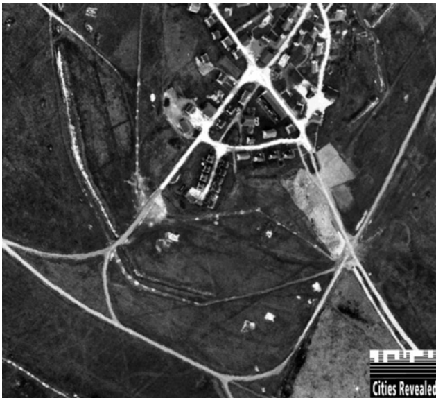
Fig. 6 Bistatic SAR image with bistatic angle \sim 50^\circ (top) along with aerial photograph of the region (Cities Revealed aerial photography © The GeoInformation Group)
