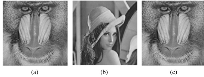
Figure 9. Encoding by system: (a) original image (b) secret image (c) steganographic image.
