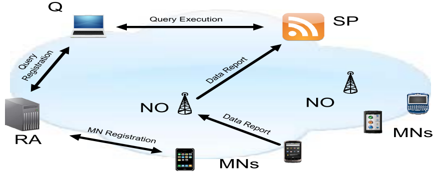
Figure 1: Privacy-Enhanced Participatory Sensing Infrastructure: Mobile Nodes (MNs) register to the Registration Authority (RA) and, subsequently, report sensed data to a Service Provider (SP). Queriers, after registering to RA, subscribe to queries offered by the SP and receive corresponding reports.
