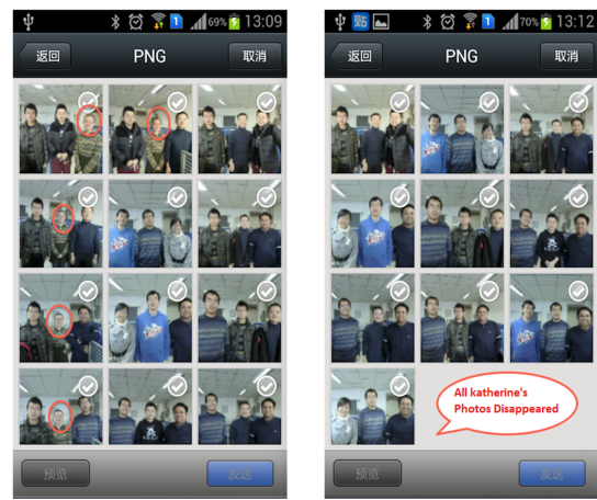
Figure 5: Case Study 2 - Photo publishing in WeChat. The screenshots show the list of photos when Alice tries to select a photo to publish in WeChat. Left: without CoDroid (using Alice’s original policy in Figure 3). Right: with CoDroid (using Alice’s co-policy specified in Figure 3.)
