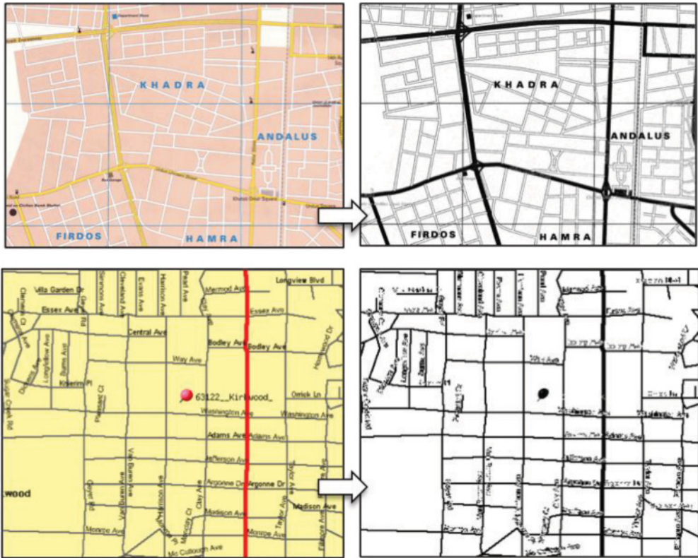
Fig. 20. Sample maps and their road layer extracted with manual grayscale histogram thresholding.
