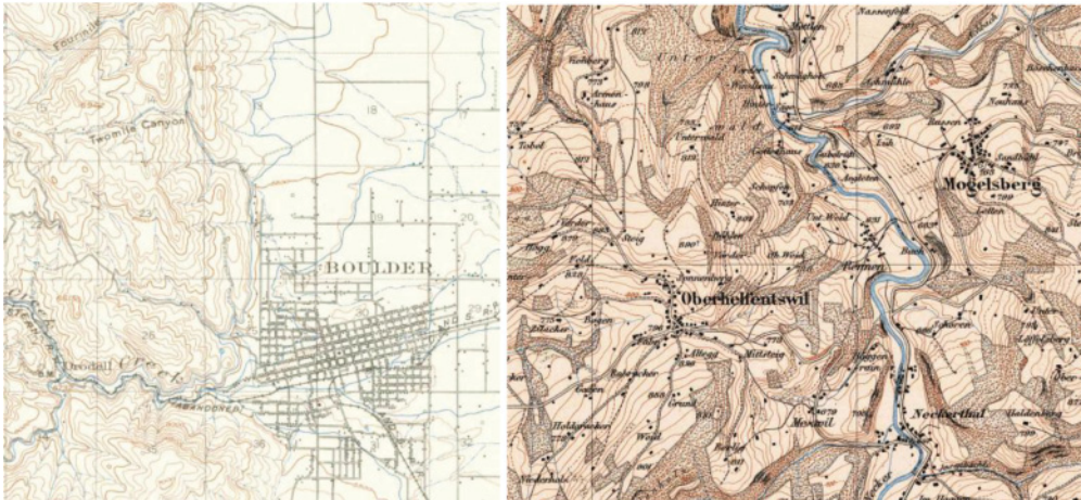
Fig. 1. Subsections of two examples of scanned (historical) maps of inferior graphical quality due to aging and bleaching effects: USGS topographic map of Boulder, Colorado (1902), at a scale of 1:62,500 (left), and Swiss National Topographic map (Siegfried map), page 220, Brunnadern (1879) at a scale of 1:25,000. Reproduced by permission of swisstopo (BA13123).
