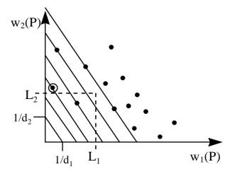
**Fig. 1.** Representation of the link weight vector w(P) of paths in two dimensions. Jaffe's scanning procedure first encounters the encircled node, which is the path with minimal length.
