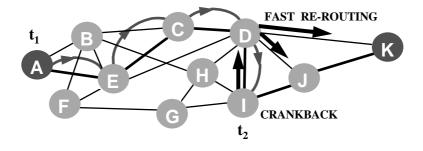
Fig. 10. Illustration of crankback and fast-rerouting.
