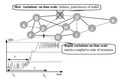
Fig. 8. Network topology changes on different time scales
