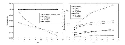
**Fig. 7.** The success rate and normalized execution time in a 100-node network, as a function of m, with the set of constraints L2.
