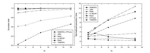
**Fig. 6.** The success rate and normalized execution time in a 100-node network, as a function of m, with the set of constraints L1.
