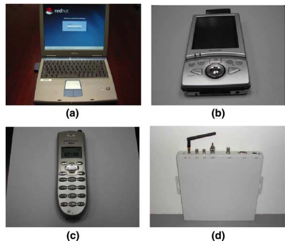
Fig. 2. Examples of mesh clients: (a) Laptop, (b) PDA, (c) Wi-Fi IP Phone and (d) Wi-Fi RFID Reader.
