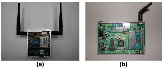
Fig. 1. Examples of mesh routers based on different embedded systems: (a) PowerPC and (b) Advanced Risc Machines (ARM).
