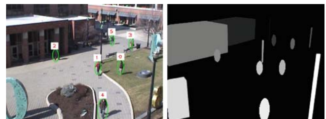
Fig. 4 Left Original frame with tracked pedestrians. Right Z-buffer (lighter shades of gray are closer to the camera)
