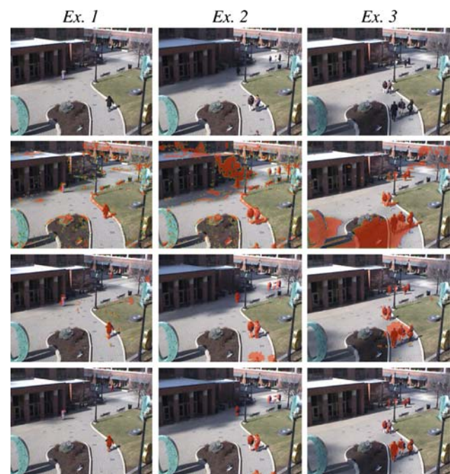
Fig. 6 Original frame (row 1). Probabilistic heatmap of the foreground (red representing higher probability) is shown using color channel only (row 2), thermal channel only (row 3), and using a combined model (row 4)
