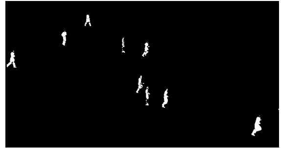
Figure 4: Foreground Segmentation: Foreground binary image after background subtraction.
