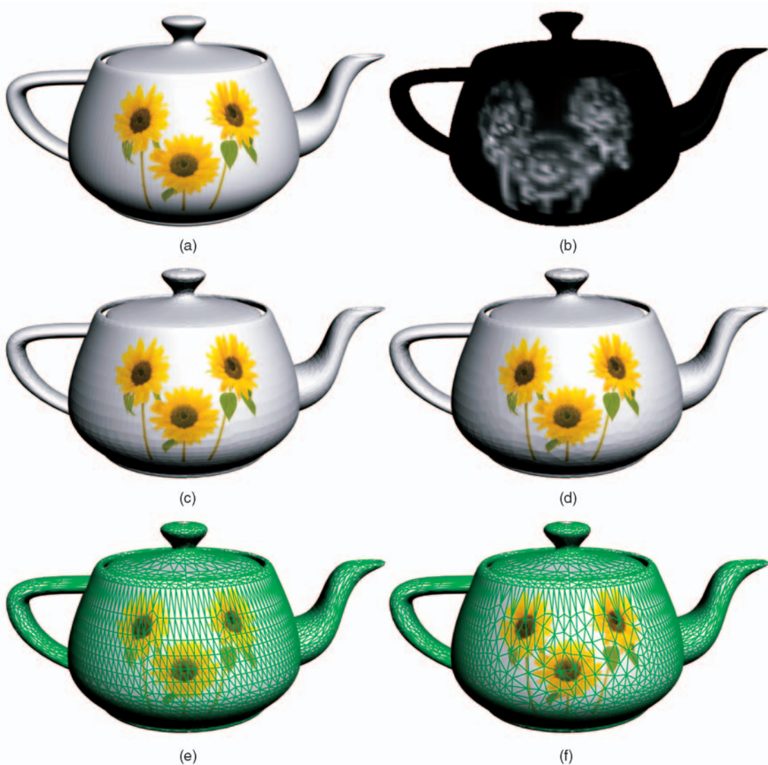
Fig. 13. (a) A rendering of the original model. (b) Masking importance map. (c) Rendered using a simplified mesh with QSlim. (d) Rendered using a simplified mesh with QSlim taking into account the masking potential of the surface light field. Both models have the same number of vertices. Their respective wireframe renderings are shown in (e) and (f).
