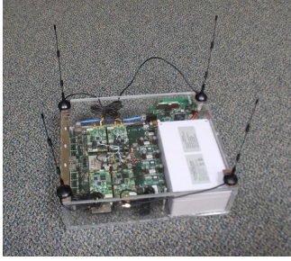
Figure 2: The autonomous ArgosMobile client is comprised of a 4-antenna WARP board, a battery, and an 802.11n bridge.
