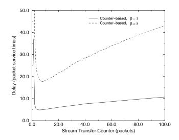
Figure 14: The mean packet delay as a function of  $T_{stc}$  for the counter-based random policy (S = 8, N = 4,  $\mu = 2.5$  pkts/s, C = 1).
