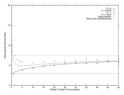
Figure 7: The mean packet delay as a function of the stream transfer time,  $T_{stt}$ , for the random selection policy. (S=4, N=2,  $\lambda$ =1 pkts/s,  $\sigma_1 = \frac{1}{50}$ ,  $\sigma_2 = \frac{1}{50}$ ,  $\mu$ =2.5 pkts/s).
