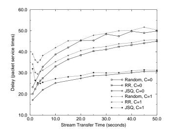
Figure 12: The mean packet delay as a function of  $T_{stt}$  for the random, round robin (RR), and JSQ policies (S = 4, N = 2,  $\lambda = 5$  pkts/s,  $\sigma_1 = \frac{1}{90}$ ,  $\sigma_2 = \frac{1}{10}$ ,  $\mu = 2.5$  pkts/s).
