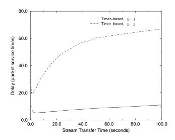
Figure 13: The mean packet delay as a function of  $T_{stt}$  for the timer-based random policy (S = 8, N = 4,  $\mu = 2.5$  pkts/s, C = 1).
