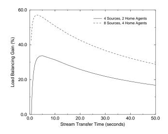
Figure 10: The percent load balancing gain, G, versus stream transfer time,  $T_{stt}$ , for different system sizes with the random selection policy ( $\lambda=1$  pkts/s,  $\sigma_1 = \frac{1}{50}$ ,  $\sigma_2 = \frac{1}{50}$ ,  $\mu=2.5$  pkts/s, C = 1).
