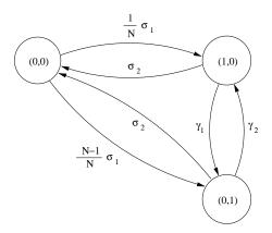
Figure 5: The modified three-state MMPP model of a source.
