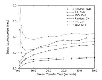
Figure 11: The mean packet delay as a function of  $T_{stt}$  for the random, round robin (RR), and JSQ policies (S = 4, N = 2,  $\lambda = 1$  pkts/s,  $\sigma_1 = \frac{1}{50}$ ,  $\sigma_2 = \frac{1}{50}$ ,  $\mu = 2.5$  pkts/s).
