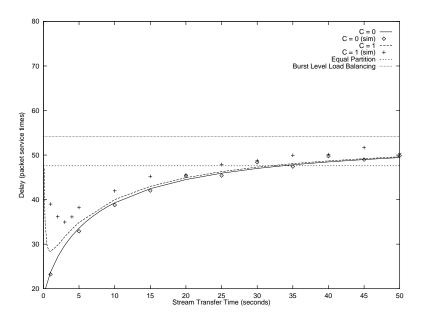
Figure 8: The mean packet delay as a function of the stream transfer time,  $T_{stt}$ , for the random selection policy. (S=4, N=2,  $\lambda$ =5 pkts/s,  $\sigma_1 = \frac{1}{90}$ ,  $\sigma_2 = \frac{1}{10}$ ,  $\mu$ =2.5 pkts/s).
