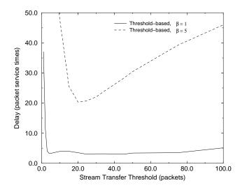
Figure 15: The mean packet delay as a function of  $T_{sth}$  for the threshold-based random policy  $(S = 8, N = 4, \mu = 2.5 \text{ pkts/s}, C = 1).$
