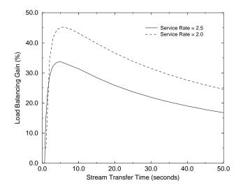
Figure 9: The percent load balancing gain, G, versus stream transfer time,  $T_{stt}$ , for different loads with the random selection policy (S=4, N=2,  $\lambda=1$  pkts/s,  $\sigma_1 = \frac{1}{50}$ ,  $\sigma_2 = \frac{1}{50}$ ,  $\mu=2.5$  pkts/s, C = 1).
