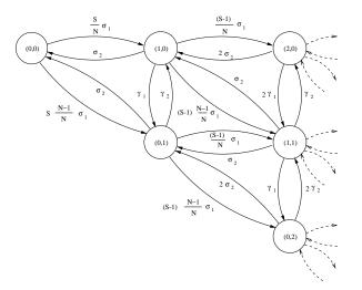
Figure 6: The state diagram of the superposition of S MMPP sources.
