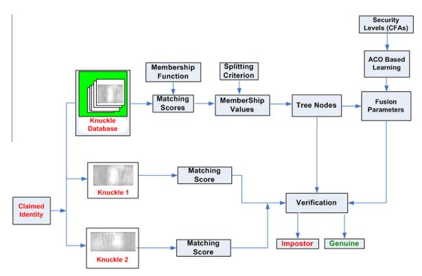
Fig. 1. Block diagram of the proposed verification system.
