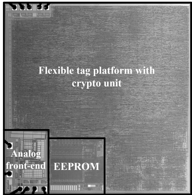
Fig. 7. Photo of the manufactured RFID tag-prototype chip.
