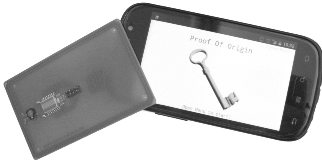
Fig. 8. Proof-of-origin application using our RFID-tag prototyping sample and the Google Nexus S mobile phone.
