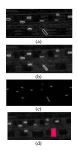
**Figure 15** Vehicle detection and incident detection results. (a) (b) Sample image of road segments. (c) Vehicle detection results, where white lines represent extracted vehicles. (d) Incident detection result.
