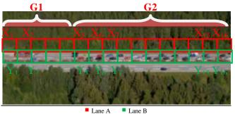
Figure 12 Traffic-flow zones added to a highway image.
