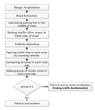
Figure 14 Flowchart for traffic bottleneck detection.
