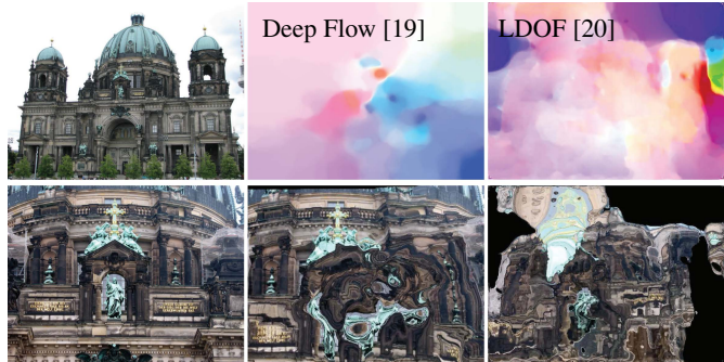
Fig. 3: An image pair with huge motion. The warp projects the second image onto the first. While this is not a difficult feature correspondence scene, the large occlusions makes it difficult for optical flow.
