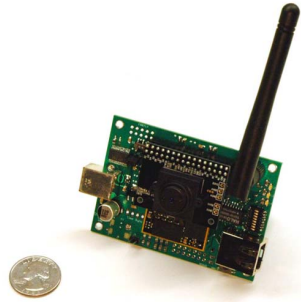
Figure 3. The DSPcam hardware.
