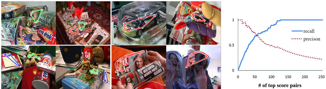
(a) Object-based image matching on the test image pairs of the ETHZ toys dataset
