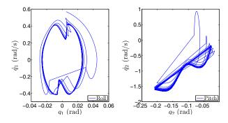
Fig. 3. Phase portraits of the closed-loop system during 50 consecutive steps of walking corresponding to the optimal solutions of (28) around the nominal output function.
