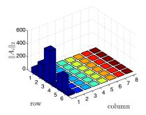
Fig. 2. Plot of the 2-norm of the sensitivity matrices versus the components of the  $6\times 8$  H matrix around the nominal output function. Here, i=row+6(column-1).
