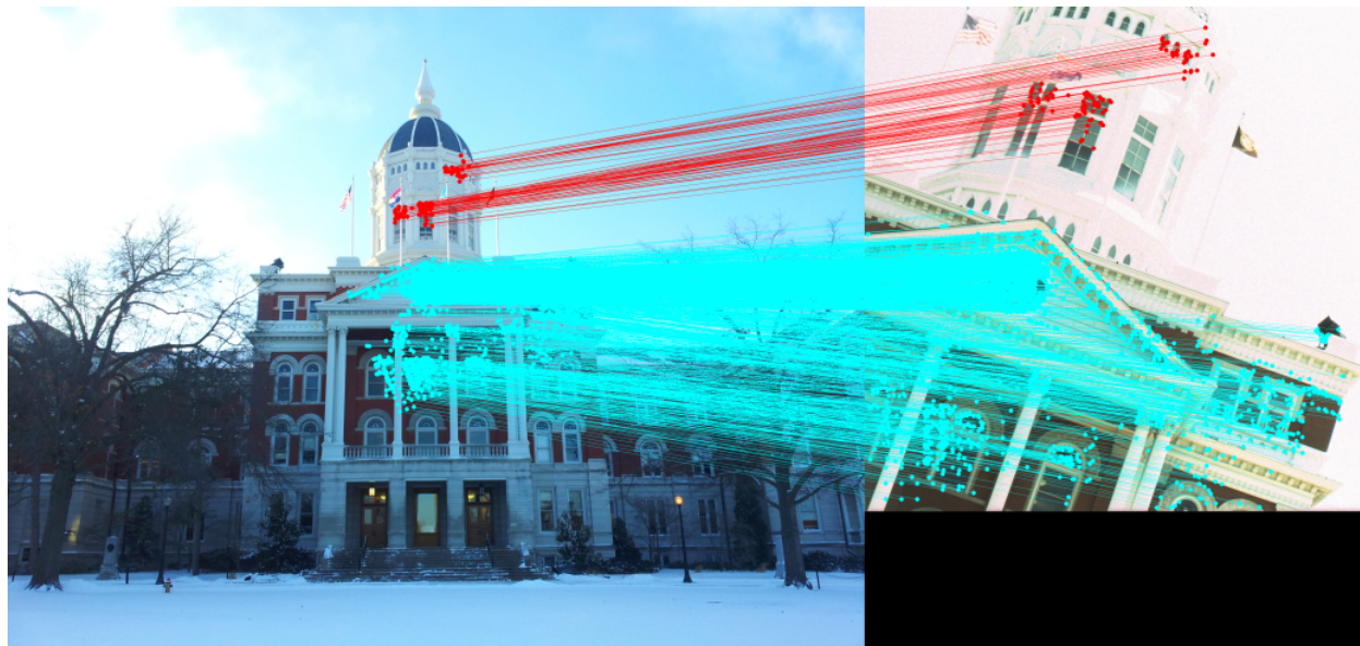
Fig. 10. Matches identified using multiple homographies. Each color corresponds to a different homography. We can see how each homography tends to find matching points in different regions and planes of the image.
