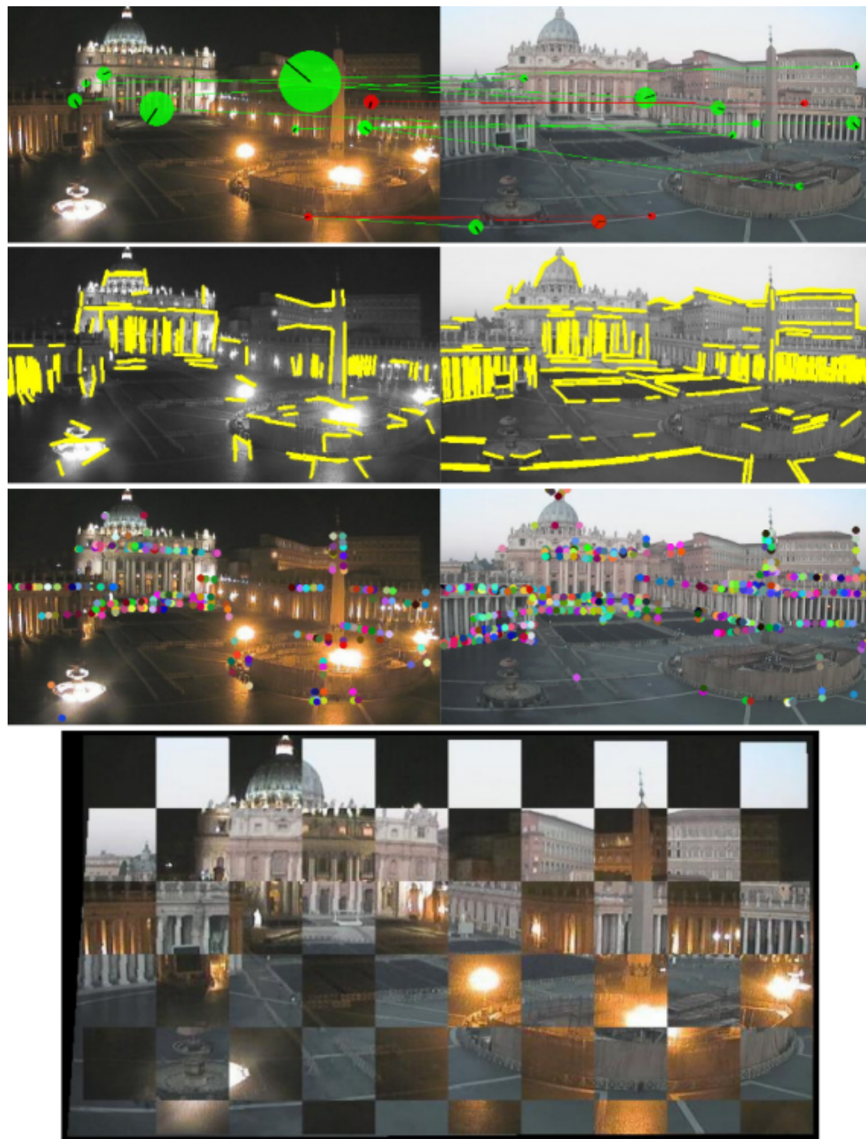
Fig. 9. Using Pseudo Corners to align a difficult image pair, called Vatican. Top : The majority of the SIFT (green) and linearly-verified (red) keypoint matches for this pair are incorrect and cannot be used to align the images. No SIFT+HOG matches were identified in this example. The relative SIFT scales are represented by the size of the circles and the features' orientations are denoted by the black lines. 2nd Row : Line segments extracted from images (shown in yellow) that are used to find Pseudo Corners. 3rd Row : Pseudo Corners identified after intersecting line segments. Bottom : Image pair is aligned using the homography calculated from the matched Pseudo Corners.
