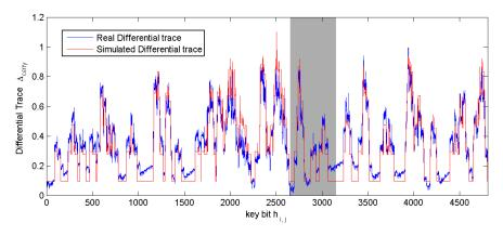
**Fig. 2.** Differential leakage trace for key rotation. The plot shows the normalized leakage (vertical axis) of both key parts  $h_{\Sigma,j} = h_0 + h_1$  over the key bit index (horizontal axis). The red(gray) line is the simulated leakage while the blue/black line is the observed leakage from the target implementation.
