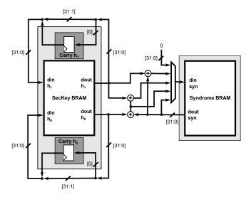
Fig. 1. Abstract block diagram of the syndrome computation circuit including key rotation as implemented in [17].
