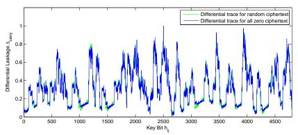
Fig. 4. Normalized differential leakage trace  $\Delta_{\text{carry}}$  for the key rotation for the bits of  $h_{\Sigma,j} = h_0 + h_1$ . Whether the ciphertext is known (green(gray) line) or all-0 (blue(black) line) has only marginal influence on the observed leakage.
