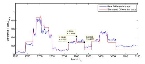
**Fig. 3.** A magnified version of Figure 2 that highlights the characteristic shape of a single set bit (center) as well as the overlap of two (right) and three (left) "adjacent" set bits.
