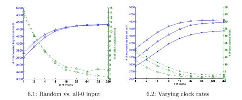
**Fig. 6.** Key bit recovery rates for recovering 0 key bits. Solid line indicates the number of recovered bits (out of 4711 zeroes, scale on left), the dashed line indicates the number of false positives (scale on right). The left figure compares known random ( $\circ$ ) vs. chosen all-0 ( $\triangle$ ) ciphertext inputs. The right figure compares the experiments for varying clock rates:  $\circ$  for 3 MHz,  $\triangle$  for 8 MHz, and \* for 16 MHz.
