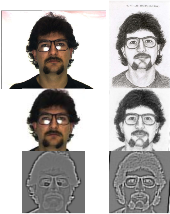
Fig. 2. Face normalization and preprocessing for a photo and sketch. Original Images (top), Normalized Images (center) and Preprocessed Images (bottom).
