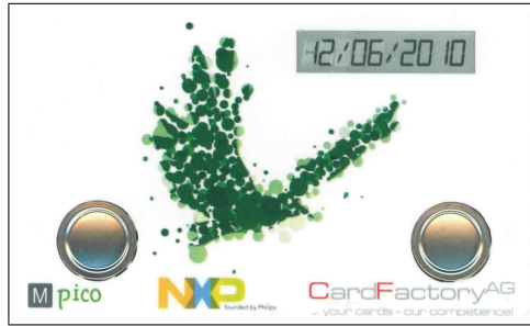
Figure 1: A Display and Button Equipped RFID Tag from NXP Semiconductors
