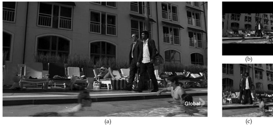
Fig. 10. Example of video retargeting: (a) original 624 \times 352 video; (b) a 120 \times 120 video by simply resizing; and (c) a 120 \times 120 video by retargeting with visual saliency.
