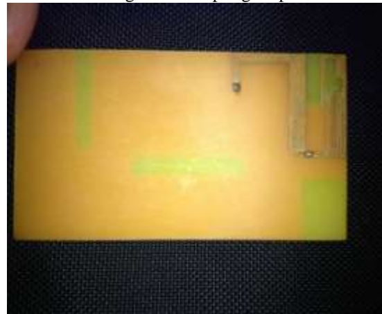
Figure 7: Resonating part of antenna
