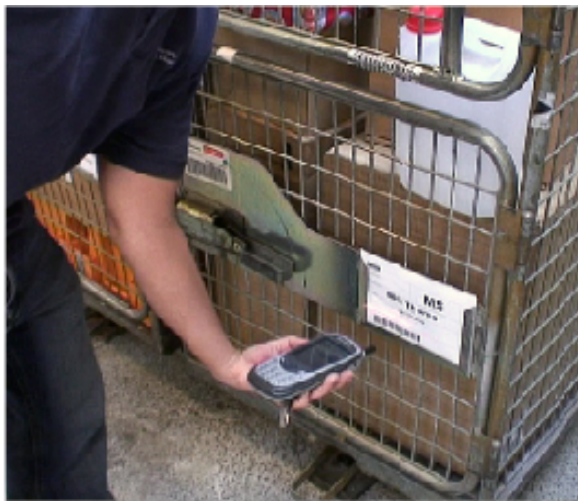
Figure 12. RFID tag placed on the container
