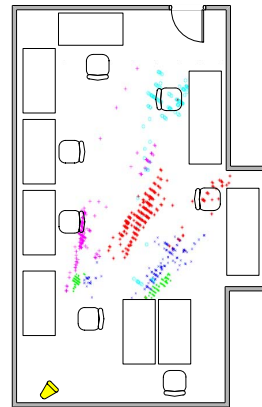
Fig. 6. The heat map of people in the office. We plot the locations of people on the schematic floor plan of the office.
