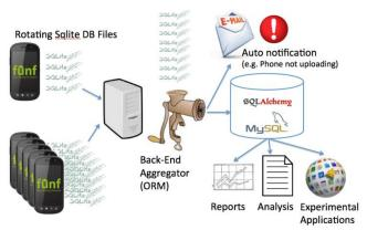
Figure 6. Back-End Data Aggregation Overview
