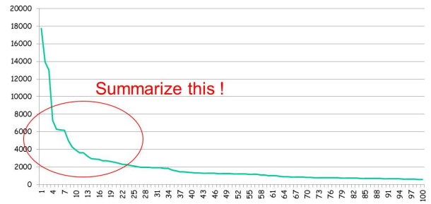
Figure 10: On the x-axis, we place different branches observed during whitebox fuzzing. On the y-axis we have the frequency of occurrence. The graph shows only the 100 first most common branches out of 3,360 total.
