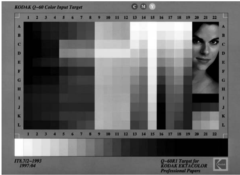
Figure 5A (See color insert following page 430) Q60 input characterization target.
