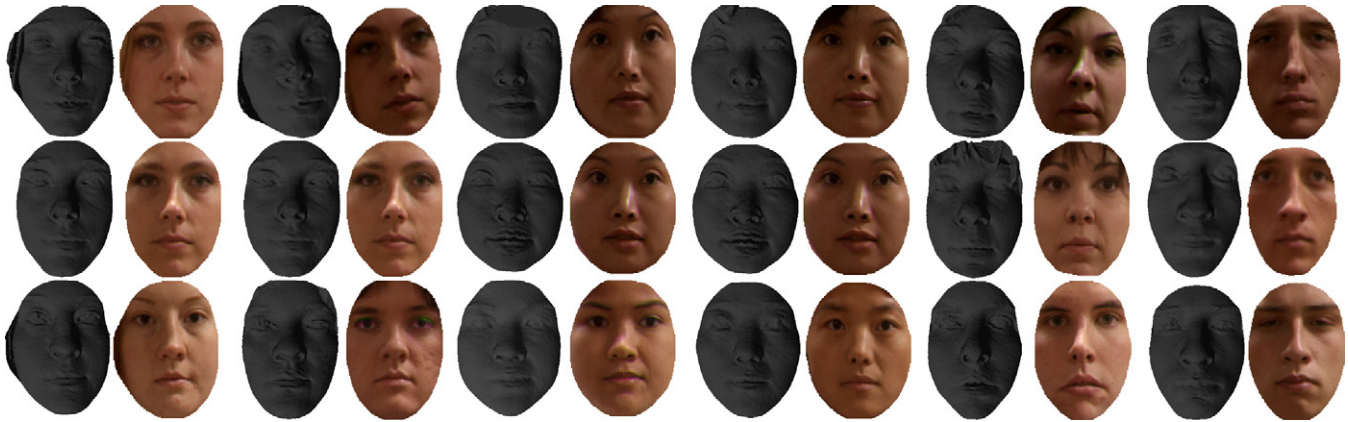
Fig. 6. Some probe faces (1st line) that were mis-recognized as gallery faces shown in the 3rd line. The correct gallery faces are shown in the middle line.
