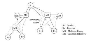
Figure 15: Hierarchical Reliable Multicasting
