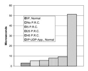
Figure 8: IP Input Processing Time for a Non-Redirected Session with Parallel Redirected Connections (P.R.C.)
