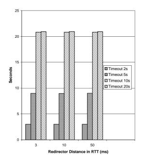
Figure 12: TCP Connection Establishment Latency for a Non-Redirectable Client with Varying Client Response Timeout
