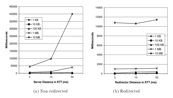
Figure 13: Bulk Transfer Time Over a TCP Connection
