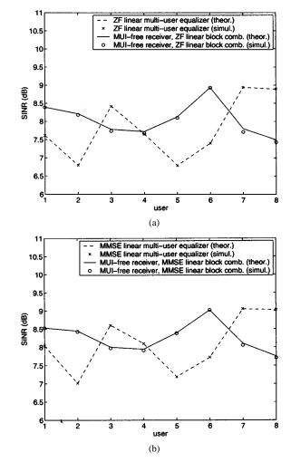
Fig. 7. Theoretical and simulated SINR as a function of the desired user for an SNR of 10 dB and an NFR of 0 dB (known channels and noise variance).
