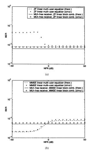
Fig. 11. Average theoretical (known channels and noise variance) and simulated (estimated channels and noise variance) BER per user as a function of the NFR for an SNR of 10 dB.
