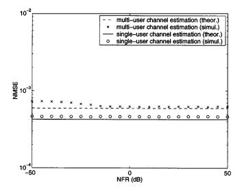
Fig. 9. Average theoretical and simulated NMSE per user of the channel estimates as a function of the NFR for an SNR of 20 dB.
