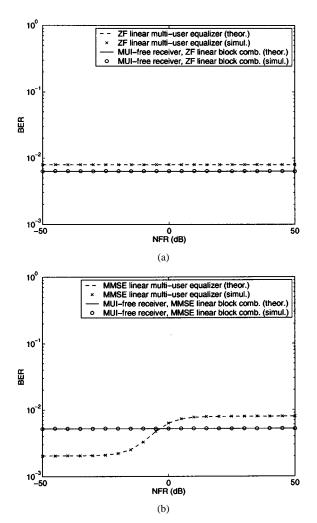
Fig. 6. Average theoretical and simulated BER per user as a function of the NFR for an SNR of 10 dB (known channels and noise variance).
