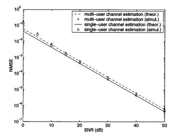
Fig. 8. Average theoretical and simulated NMSE per user of the channel estimates as a function of the SNR for an NFR of 0 dB.
