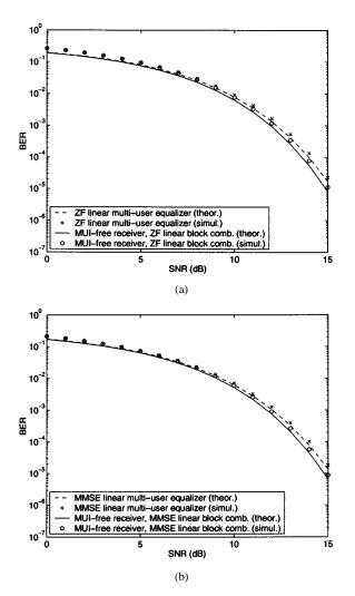
Fig. 10. Average theoretical (known channels and noise variance) and simulated (estimated channels and noise variance) BER per user as a function of the SNR for an NFR of 0 dB.
