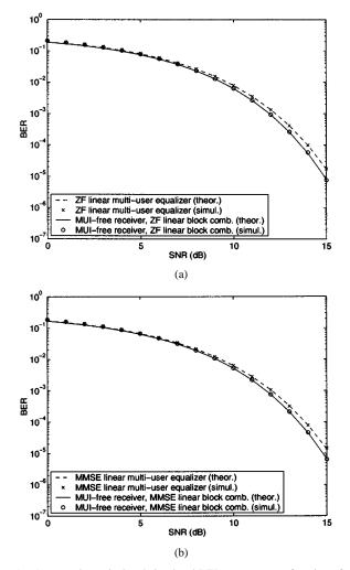
Fig. 5. Average theoretical and simulated BER per user as a function of the SNR for an NFR of 0 dB (known channels and noise variance).
