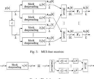
Fig. 4. Block despreading.
