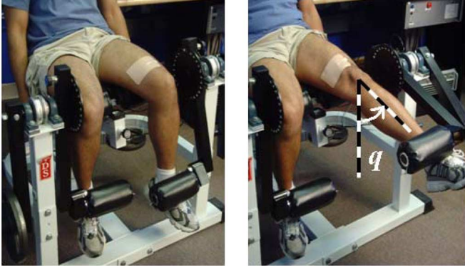
Fig. 1. In left image the subject's left leg is in relaxed state. The right image shows the left leg during stimulation. The angle q(t) is measured with respect to the vertical line as shown.
