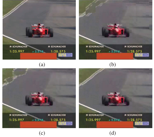
Fig. 5. The interpolated results of frame 56 of FORMULA 1 sequence using a) the original frame 56, (b) direct MCFI (PSNR: 29.68dB), (c) the method in [8] without color consideration (PSNR: 29.58dB), and (d) the method in [8] with color consideration (PSNR: 31.12dB), respectively.
