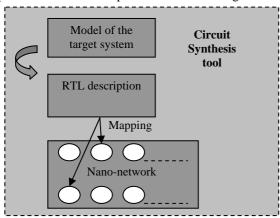
Figure 6: Circuit synthesis tool
