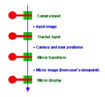
Figure 6. Mirror simulation application graph.
