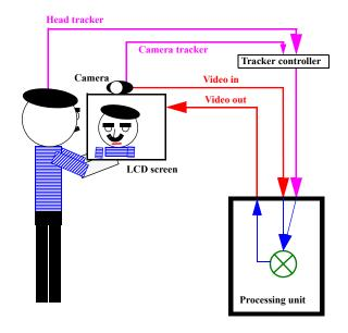
Figure 1. Handheld mirror simulation system.
