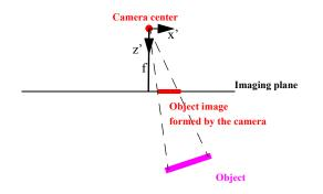
Figure 3. Pinhole camera geometry.
