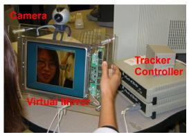
Figure 7. Handheld mirror device.
