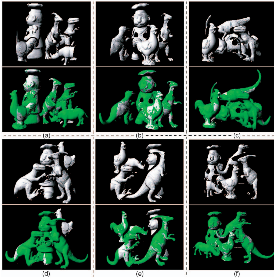
Fig. 20. Recognition results of our algorithm on six real scenes. These scenes do not have any background due of the limited range of the Minolta scanner. All objects are correctly recognized except for the chicken in (d) and the chef in (e).
