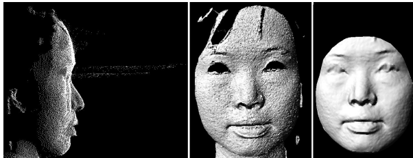
Fig. 1. (Left) A 3D pointcloud of a face shows spikes. (Center) The same face rendered as a shaded view to show noise. (Right) Shaded view after preprocessing.
