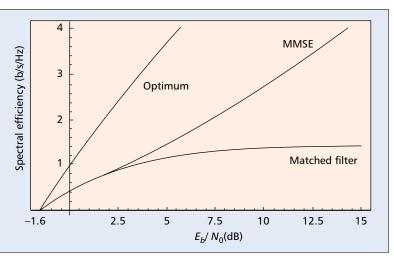
**Figure 2.** *CDMA* spectral efficiencies with optimum coding-spreading trade-off.
