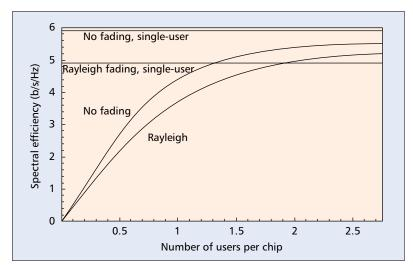
Figure 1. Optimum CDMA spectral efficiency at an energy per bit per thermal noise level of 10 dB.
