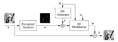
Fig. 2. Generation of a spread spectrum watermark.
