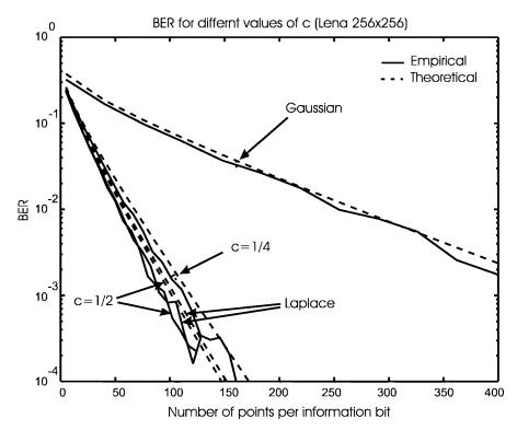
Fig. 18. BER versus pulse size for "Lena" ( $256 \times 256$ ).
