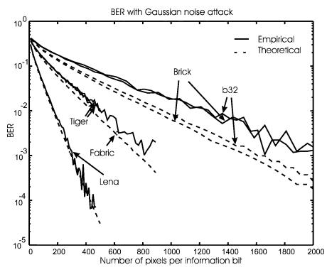
Fig. 9. BER with additive Gaussian noise attack.
