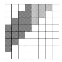
Fig. 16. DCT coefficients where the watermark is embedded.
