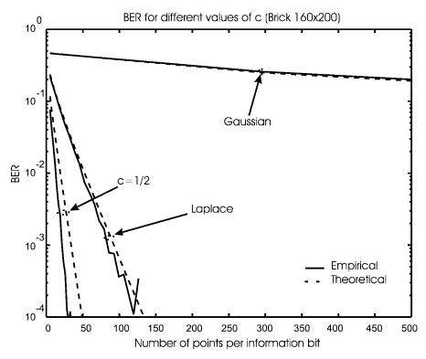
Fig. 19. BER versus pulse size for "Brick" (160  $\times$  200).
