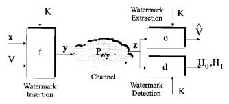
Fig. 1. General model of a watermarking system.
