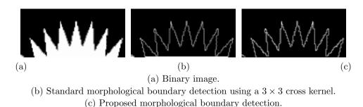
Fig. 7. Comparison: proposed boundary detection is preserve better details that the standard (with a  $3 \times 3$  cross) morphological boundary detection. In addition, the proposed detection is significantly faster.
