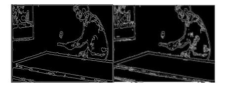
(c) Canny boundary detection: boundaries with gaps, point linking is necessary.
