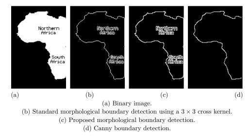
Fig. 8. Boundary detection comparison. Note the shape distortion when using Canny detector. The proposed detection gives more accurate results than the standard morphological detector using a  $3 \times 3$  cross kernel.
