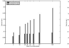
(a) Cost of proposed versus standard erosion.
