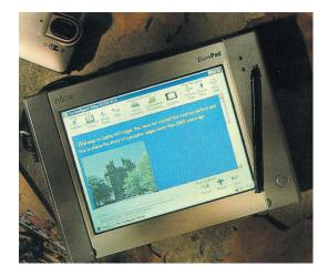
to enable viewing in bright sunlight, has a Pentium 166 MMX processor, and weighs approximately 850 grams.
