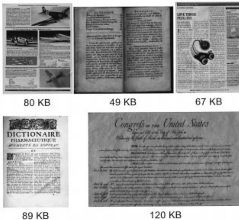
Fig. 34. Document images with file sizes after compression in the DJVU format at 300 dpi.
