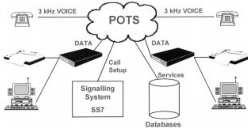
Fig. 3. The POTS network with signaling, service-oriented data bases, and connections for facsimile devices and PC's via voice-band modems.
